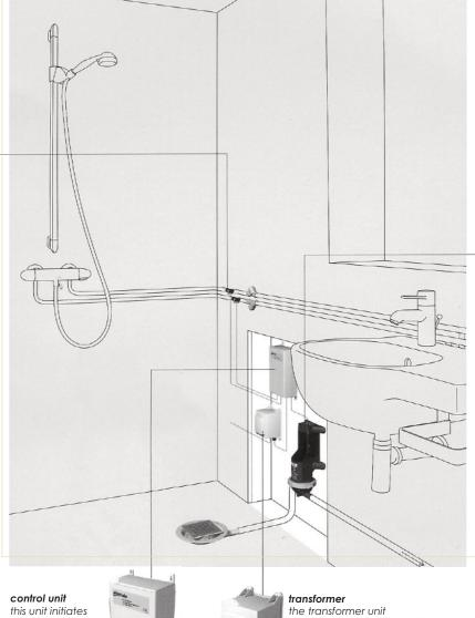
the transformer unit converts the mains electricity supply (230v A.C.) to the low voltage DC supply required for the pump in domestic installations.
